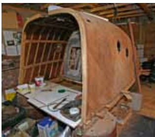
ABOVE The new engine canopy in build.
