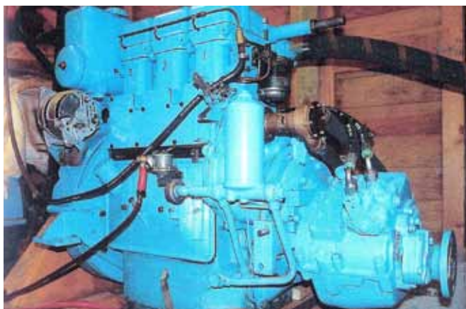
BELOW The reconditioned Lister HW3M engine ready for installation in Anne Allen.
